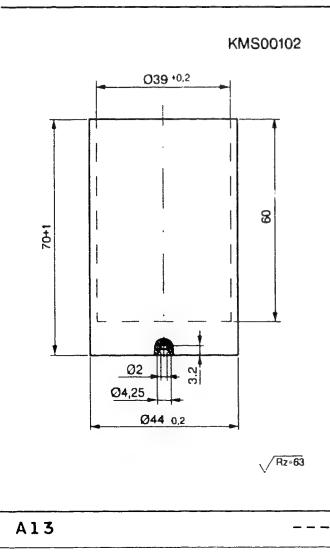
TESTERS, FIXTURES, TOOLS Thrust piece for pressing deep-groove ball bearing onto bearing end plate: (improvisation)
